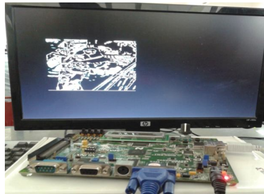
Fig 5: FPGA Output For Blurred Filter
